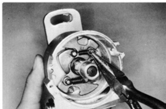
Fig. 8-94 Remove Governor Spring
